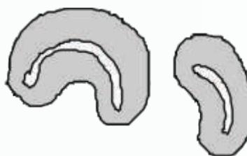
Figure 2.3 Cross-section of cotton fibres
