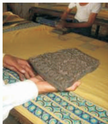
Figure 2.25 Block printing process
