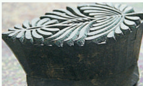
Figure 2.24 A wooden block for block printing
