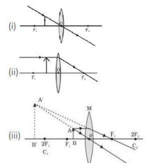
The image is virtual, erect and larger than the object.
