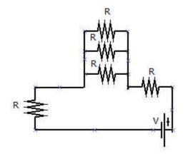
Q. 5. In the circuit shown below, calculate the net resistance of the circuit.
