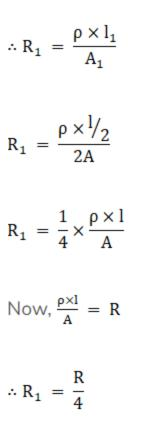
Thus, we can conclude that the new resistance of the wire when the area of wire is doublead and length is haved become the initial resistance.
