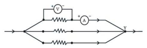
• We will close the switch and note the readings. Similarly, we will switch the position of voltmeter to resistances  $R_2$  and  $R_3$  and observe the readings.
