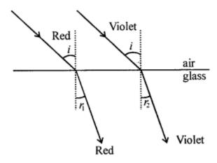
The two refracted rays inside glass are not parallel. Because the refractive index of glass is less for Red light,
