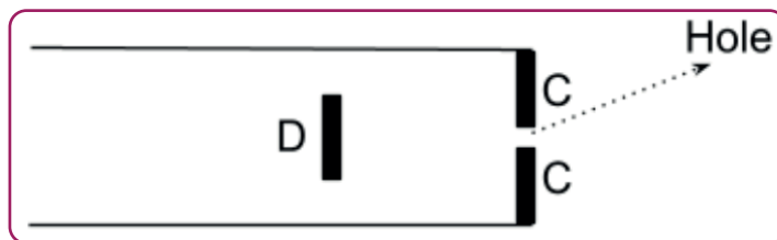
Fig. 5.22, Hole in the primary element of a reflecting telescope
