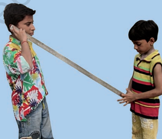
Fig. 13.12 : Sound travelling through a metre scale
