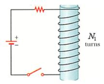
This result is easily obtained by integrating Ampère's law over a rectangular loop whose long sides run parallel to the axis of the solenoid, one inside the solenoid, and the other outside, and whose short sides run perpendicular to the axis. The magnetic flux though each turn of the loop is
