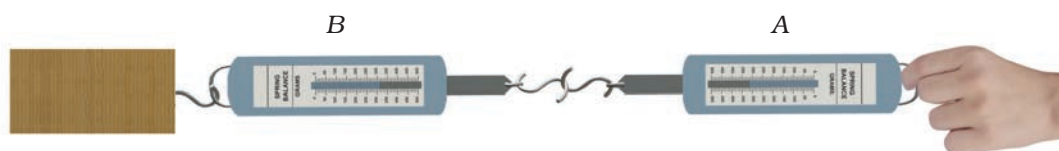
Fig. 34.1 : Action and reaction forces are equal and opposite
