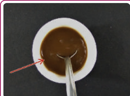
Fig. 1.12, Add fine soil into a small cup of water and stir it well
