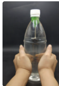
Fig. 5.9, Once you let go, it floats back up again. You can vary the pressure applied to make it float at various heights in the bottle.
