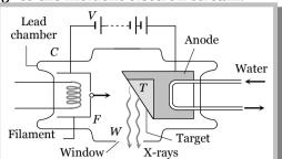
The filament is heated by pass applied between the target and cath highly energetic electrons are focus
