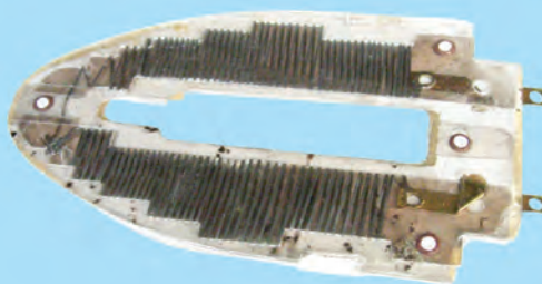
Fig. 14.11 Element of electric iron
