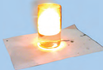
Fig. 4.5 : Reaction of sodium with water
