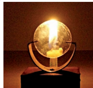
Virtual image formed by the convex lens
