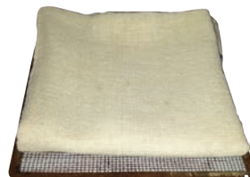
Figure 56.3 Spreading of wet pulp paste on the muslin cloth
