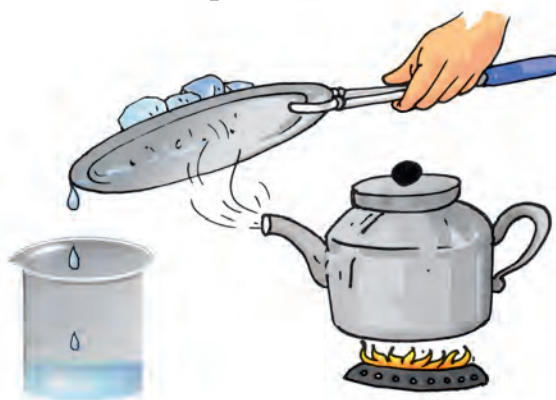
Fig. 5.13 Evaporation and condensation
