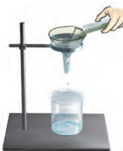
Fig. 5.10 Filtration using a filter paper
