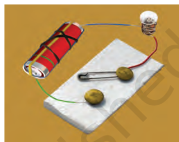
Fig 12.9 An electric circuit with a switch
