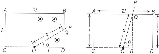
the rod  $OP$  will make contact with the side  $BD$ . Let the length  $OQ$  of the contact at sometime  $t$  such that  $0 < t < \frac{\pi}{4\omega}$  or  $0 < t < \frac{T}{8}$  be  $x$ . The flux through the area  $ODQ$  is
