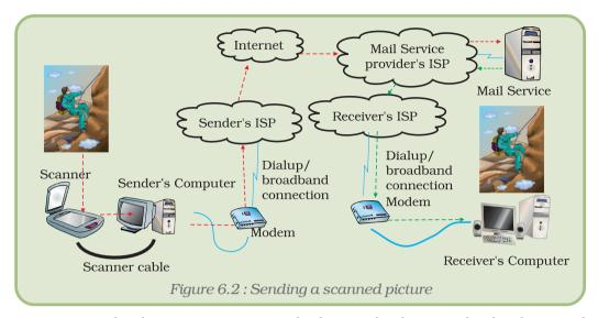
Apparently this operation may look simple, but in the background there are many interconnected devices and networks that are involved. At various stages, our data (picture) is converted into various forms until it reaches the final destination.
