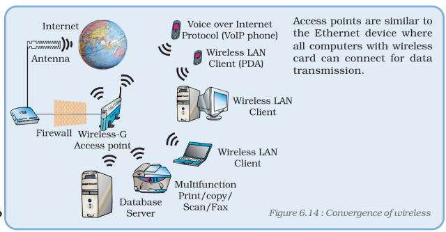
Wireless LAN, WiFi and WiMax are few such technologies which provide high speed data communication over wireless networks. Computer systems are designed with built-in wireless interface cards which can connect to any type of wireless networks. In wireless network, computers are connected to the nearest available access point.
