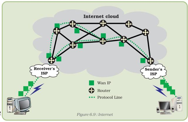
as IP address/**domain name** respectively. The computer sends the IP packet directly to the connected IP network. In the Internet the packets are forwarded from one network to other as per the destination address till it reaches the receiver.
