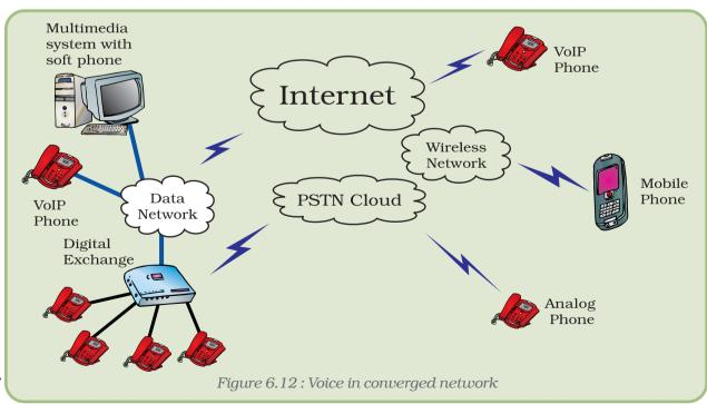
well as with multimedia computer connected with the Internet. Instant messages can be sent from a computer to a mobile phone. Devices from one network can communicate with devices from other network through gateways. Gateways are communication devices used to interface different networks. Manufacturers are developing multipurpose plug and play devices which can be connected anywhere at any time.
