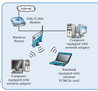
Wireless Network: Communication medium where devices are not connected through any cables, but through radio waves. Mostly used for connecting areas where the users are always mobile or it is not possible to lay cables.
