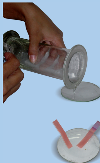
Fig. 4.4 (b) : Testing of solution with litmus papers
