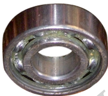
Fig. 12.16 : Ball bearings reduce friction
