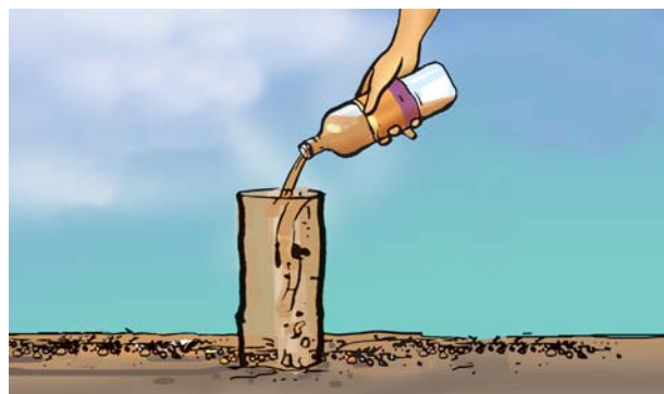
Fig. 9.5 Measuring rate of percolation
