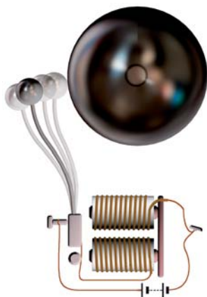
Fig. 14. 20 Circuit of an electric bell
