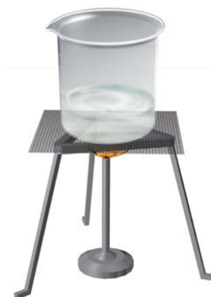
Fig. 5.11 Heating a beaker containing salt water and disappear completely? Now, add two spoons of salt to water in another beaker and stir it well. Do you see any change in the colour of water? Can you see any salt in the beaker, after stirring? Heat the beaker containing the salt water (Fig. 5.11). Let the water boil away. What is left in the beaker?
