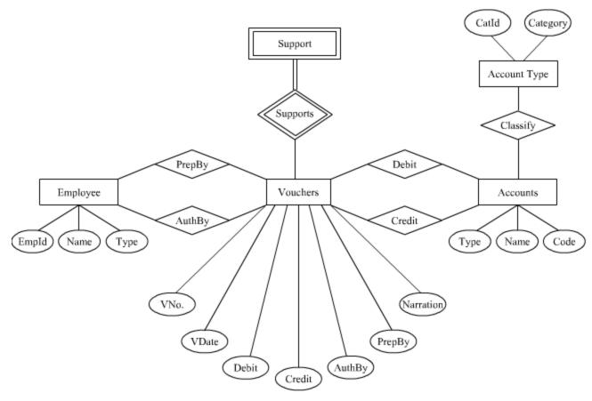
In the above diagram, the rectangular boxes are used to represent entities. The diamond shaped boxes are used to describe the relation type between the two entities. The double lined rectangular boxes are used to show the weak entities. The double-lined diamond shaped box is used to describe the identifying relationship type. In ovals, attribute names are enclosed and attached to their respective entity type through the straight lines.
