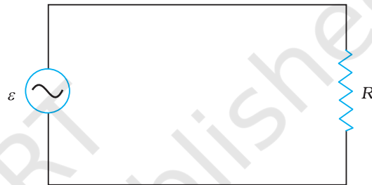
FIGURE 7.1 AC voltage applied to a resistor.
