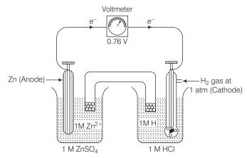
The EMF of the cell comes out to be 0.76 V. (reading of voltmeter is 0.76 V).  $\rm Zn^{2+}$  /  $\rm Zn\,couple$  acts as anode and SHE acts as cathode.
