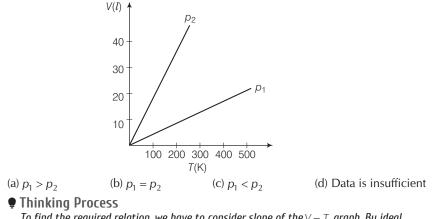
To find the required relation, we have to consider slope of the V - T graph. By ideal gas equation, the slope of V-T curve is V/T = nR/p. This imply that greater the slope, smaller the pressure and vice-versa.
