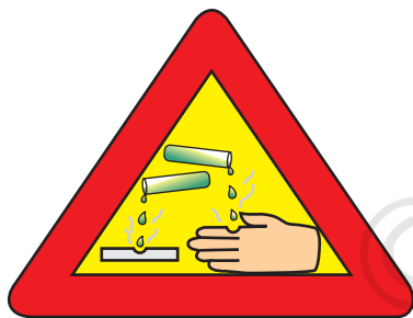
Figure 2.5 Warning sign displayed on containers containing concentrated acids and bases
