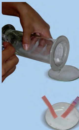
Fig. 4.4 (b) : Testing of solution with litmus papers
