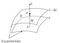
Here, the figure electric field is always remain in the direction in which the potential decreases steepest. Its magnitude is given by the change in the magnitude of potential per unit displacement normal to the equipotential surface at the point.
