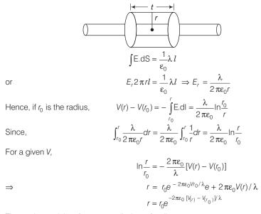
The equipotential surfaces are cylinders of radius.
