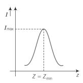
As frequency (v) increases, Z decreases and at certain value of frequency know as resonant frequency (v<sub>0</sub>), impedance Z is minimum that is  $Z_{\min} = R$  current varies inversely with impedance and at  $Z_{\min}$  current is maximum.
