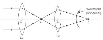
The point image  $I_1$ , due to  $L_1$  is at the focal point. Now, due to the converging lense  $L_2$ , let final image formed is I which is point image, hence the wavefront for this image will be of spherical symmetry.
