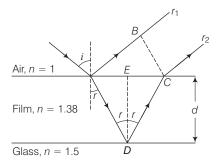
Refractive index of film = 1.38 and refractive index of glass = 1.5. Given,  $\lambda = 5500 \, \text{Å}$ .
