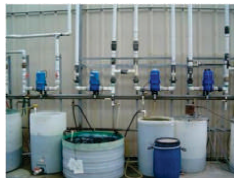
Tanks of fertigation system containing nutrient solutions
