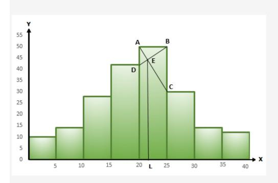
In the highest rectangle which represents modal class draw two lines AC and BD intersecting at E. From E, draw a perpendicular to x-axis meeting at L. Value of L is the mode. Hence, mode = 21.5
