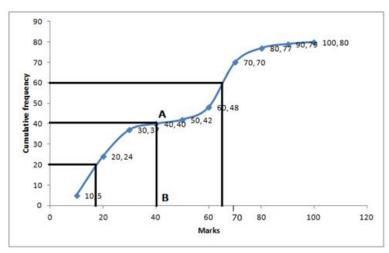
(i) Median = Through  $40^{th}$  term mark draw a line parallel to the x-axis which meets the curve at A. From A, draw a perpendicular to x-axis which meets it at B.
