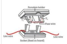
A fuse is connected with each electrical appliance to safeguard it from the flow of excessive current through it.
