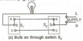
Similarly if the bulb is in on position as shown in Fig. (b) or (c), one can switch off the bulb either from the switch  $S_1$  or the switch  $S_2$ .
