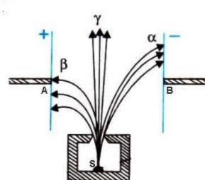
(b) The radioactive substances are kept in thick lead containers with a very narrow opening, so as to stop radiations coming out from other directions because they may cause biological damage.
