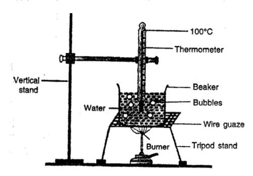
Record the temperature after evefy minute. Temperature rises and as it reaches 100°C water starts boiling. Though heat is being supplied temperature does not rise i.e. it remains constant at 100°C and bubbles formed are seen. Thus, boiling point of water is 100°C and at boiling point heat supplied is absorbed by water at constant temperature. Because this heat is being used to change every molecule of water into vapours
