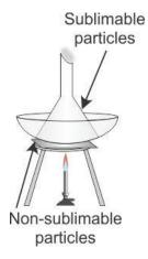
Working- A mixture of sublimable and non-sublimable substances is placed on an evaporating dish which is covered with an inverted flask plugged with cotton. On heating, the sublimable component evaporates and further condenses on the sides of the flask and the non-sublimable component remains in the evaporating dish. Example- Sublimation can be used for the separation of ammonium chloride and sodium chloride in the laboratory.
