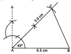
(ii) At A, draw a ray making an angle of 45° and cut off AC = 5.8 cm
