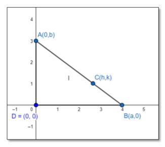
Here line segment AB represents the rod of length I also  $\triangle$ ADB formed is a right triangle. Coordinates of A and B are assumed to be (0,b) and (a,0) respectively.
