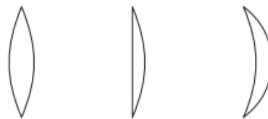
(a) Double convex lens (b) Plano-convex lens (c) Concavo-convex lens
