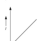
V - I graph for an ohmic conductor
