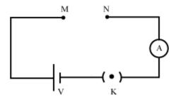
Connect copper wire of case (i) between the open points M and N, and note the readings in the ammeter. The reading will give you the amount of current flowing through the copper wire.
