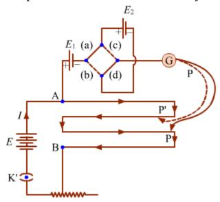
When the keys (a) and (b) are closed and keys (c) and (d) are opened, the cells are connected as the total emf of the combination becomes  $E_1+E_2$ .
