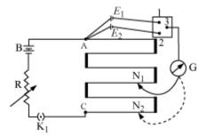
In the above figure you see that a current I flows through the wire which can be varied by a variable resistance (rheostat, R) in the circuit. Since the wire is uniform, the potential difference between A and any point at a distance l from A is  $\varepsilon(l) = \varphi l$ , where  $\varphi$  is the potential drop per unit length.
