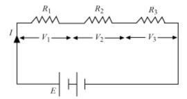
Equivalent resistance,  $R_S = R_1 + R_2 + R_3$
