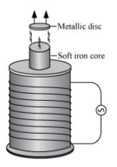
**Experiment** – Introduce a soft iron core inside a solenoid and connect it to a source of alternating *emf*. Place a metallic disc over the cross-sectional face of the soft iron core. As the circuit is switched on, the metallic disc is thrown up into the air.
