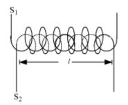
Consider two long solenoids  $S_1$  and  $S_2$  of same length l, such that solenoid  $S_2$  surrounds solenoid  $S_1$  completely.
