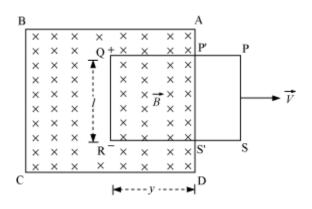
Consider that at any time *t*, the part P'Q = S'R = y of the coil is inside the magnetic field. Let *l* be the length of the arm of the coil.
