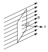
• Unit of magnetic flux – The SI unit of magnetic flux is Weber (Wb). One Weber is the amount of magnetic flux over an area of 1 m<sup>2</sup> held normal to a uniform magnetic field of one tesla.
