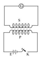
• Coefficient of mutual induction – Consider two coils *P* and *S*. Suppose that a current *I* is flowing through the coil *P* at any instant i.e.,
