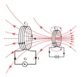
When the bar magnet is replaced by a second coil  $C_2$ , connected to a battery, the steady current in coil  $C_2$  produces a steady magnetic field. As coil  $C_2$  is moved towards coil  $C_1$ , the galvanometer shows a deflection. This indicates that electric current is induced in coil  $C_1$ . When  $C_2$  is moved away, the galvanometer shows a deflection again, but this time in the opposite direction. The deflection lasts as long as coil  $C_2$  is in motion.
