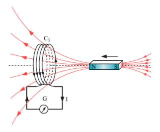
The relative motion between the magnet and the coil generates electric current in the coil. The current so generated is called induced current.
