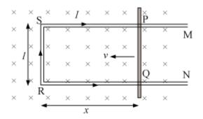
Let '*r*' be the resistance of movable arm PQ of the rectangular conductor. We assume that the remaining arms QR, RS, and SP have negligible resistances compared to *r*. Thus, the overall resistance of the rectangular loop is *r* and this does not change as PQ is moved.
