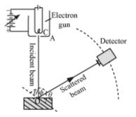
The electrons are scattered in all directions by the atoms in the crystal and its intensity in a given direction is found by the use of a detector.
