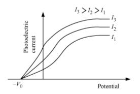
The minimum negative potential  $V_0$  given to plate A with respect to plate C at which the photoelectric current becomes zero is called stopping potential or cut off potential. If e is the charge on the photoelectron, then
