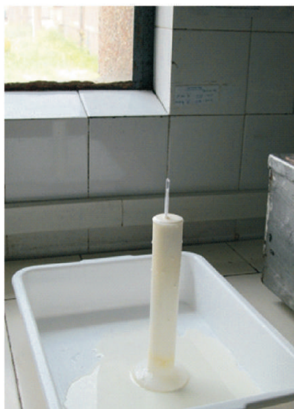
Fig.2.1. Measurement of density of milk using lactometer
