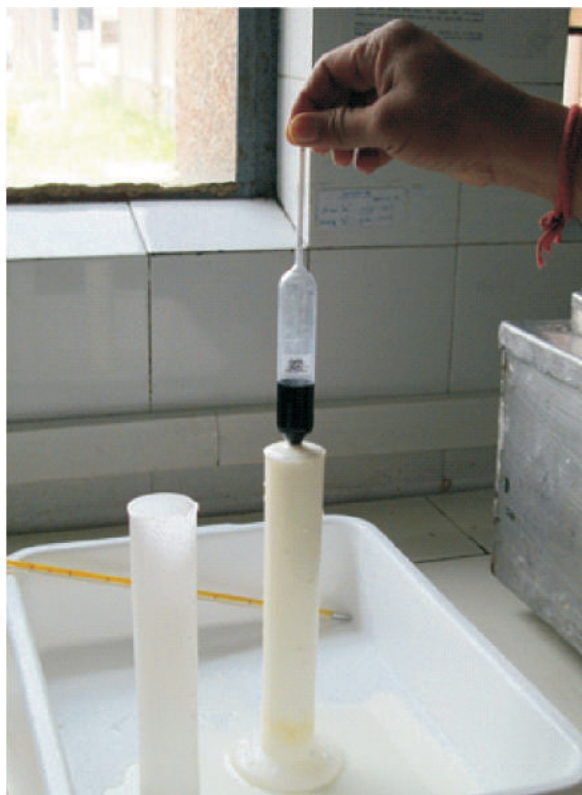
Fig.2.1. Measurement of density of milk using lactometer
