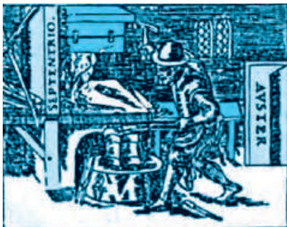
FIGURE 5.15 A blacksmith forging a permanent magnet by striking a red-hot rod of iron kept in the north-south direction with a hammer. The sketch is recreated from an illustration in De Magnete , a work published in 1600 and authored by William Gilbert, the court physician to Queen Elizabeth of England.
