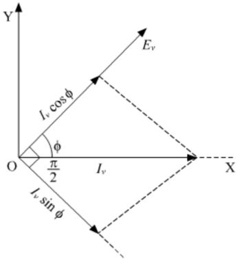
The component  $I_{\rm V}$  sin $\varphi$  makes no contribution to the consumption of power in the a.c. circuit. Hence, it is known as wattless current.
