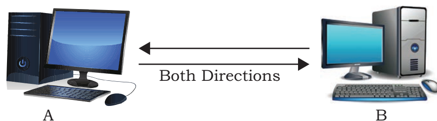
Figure 11.5: Full duplex transmission of data
