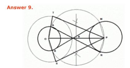
Steps of construction of transverse common tangent:
